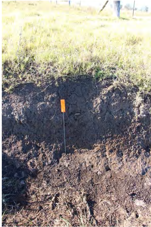
Plate 1 Hydro-AS04-14: In-situ bifacial silicified tuff core (to right of flag - flag is 50 cm long)
